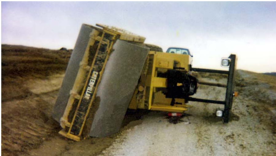
Figure 1. The overturned drum roller
