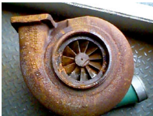
Figure 1. The rusted turbocharger
