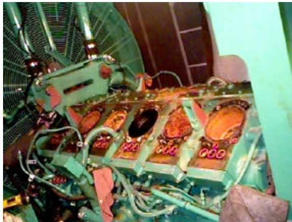
Figure 2. Damaged cylinder bank
