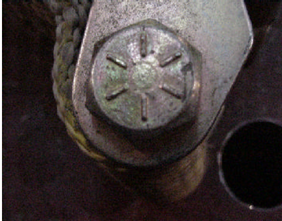
Figure 2: Close-up of suspect/counterfeit bolt
