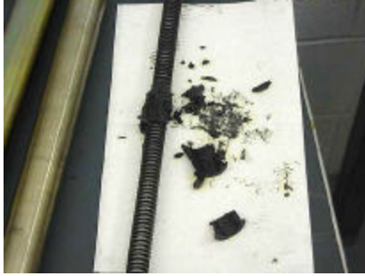
Figure 3. The failed bushing
