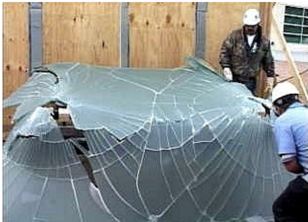
Figure 1: Shattered glass projection screen lying on top of cart
