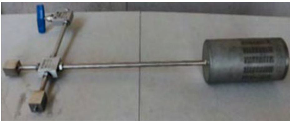
Figure 47. Assembly used for fire testing of plutonium storage containers associated with the Surplus Plutonium Disposition Project.
