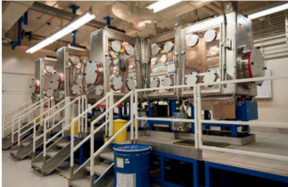
Figure 15. Centralized waste processing gloveboxes in the LLNL Plutonium Facility.
