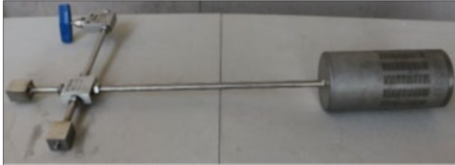
Figure 20. Assembly Used for Fire Testing of Plutonium Storage Containers
