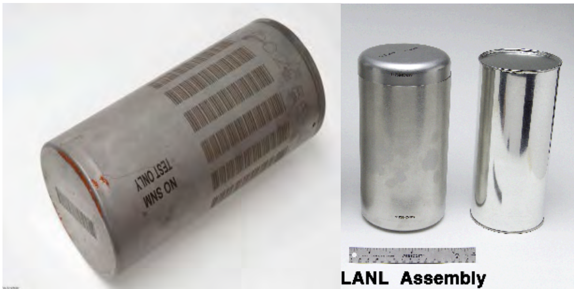
Figure A-2. Flowform container configuration, example from LANL. From left to right, these are the outer, inner, and convenience containers.
