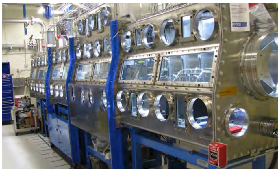
Figure 10. Glovebox Line 1 of the Recovery Glovebox Line.
