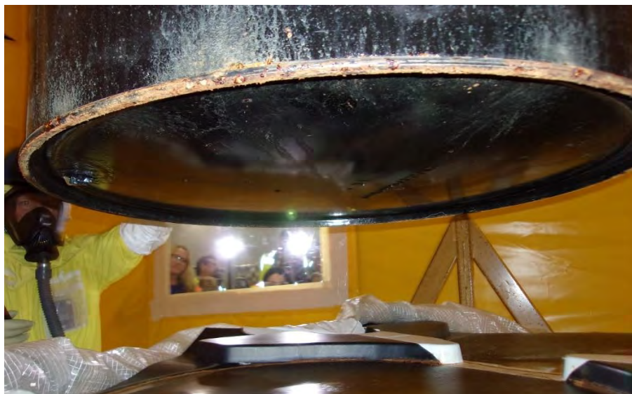
Figure 15. Areas of corrosion, paint bubbles, and fluid under a 100-gallon drum from TRUPACT-II 148.
