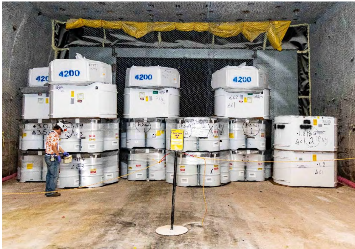
Figure 17. Waste containers in an active waste panel at WIPP.
