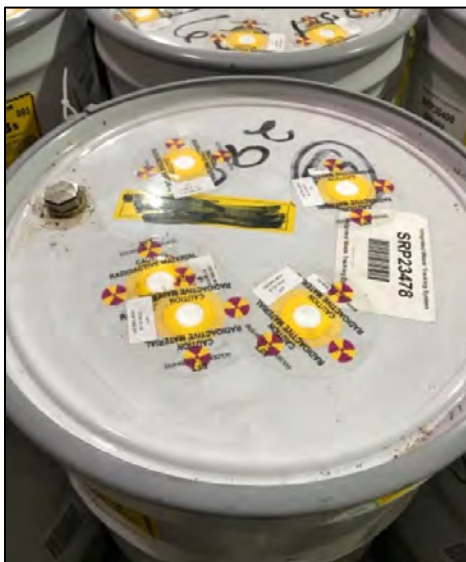
Figure 4. Waste drum at INL with multiple vents, with adhesive filters covering the vents
