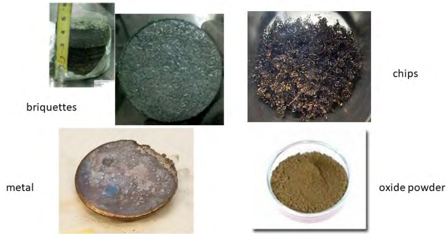
Figure 1. Uranium Material Forms at Y-12.
