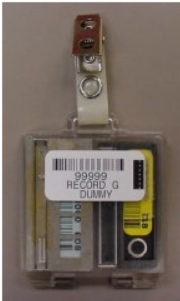
Figure 15. Thermoluminescent Dosimeter to Monitor External Radiation Dose
