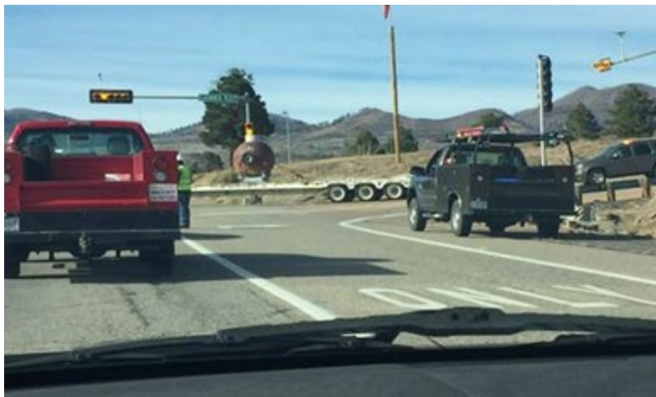
Figure 3. Rolling Roadblock During Onsite Transportation of Confinement Vessel at Los Alamos National Laboratory
