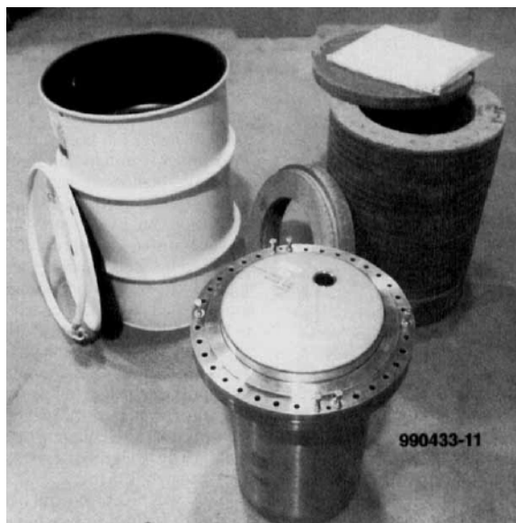
Figure 1. Pit Storage Container with Packing Material and Sealed Insert
