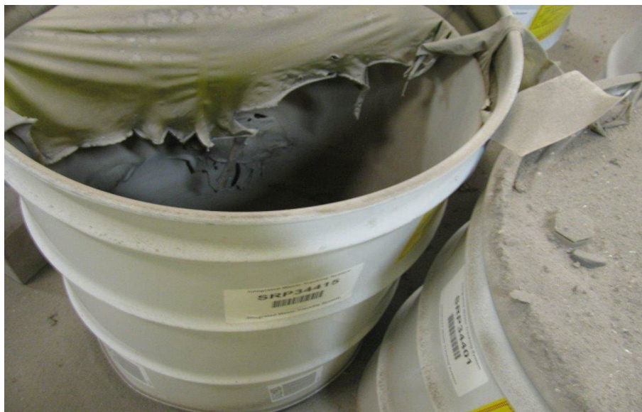
Ruptured Drum in ARP-V at Idaho National Laboratory
