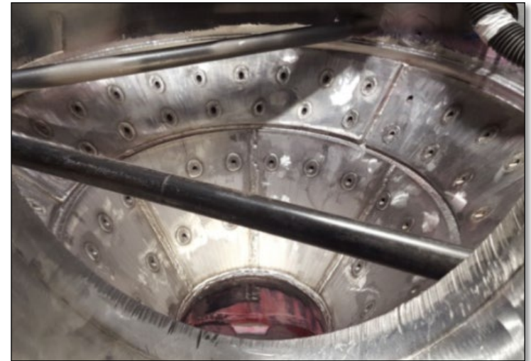
Denitration Mineralization Reformer Double Plenum
