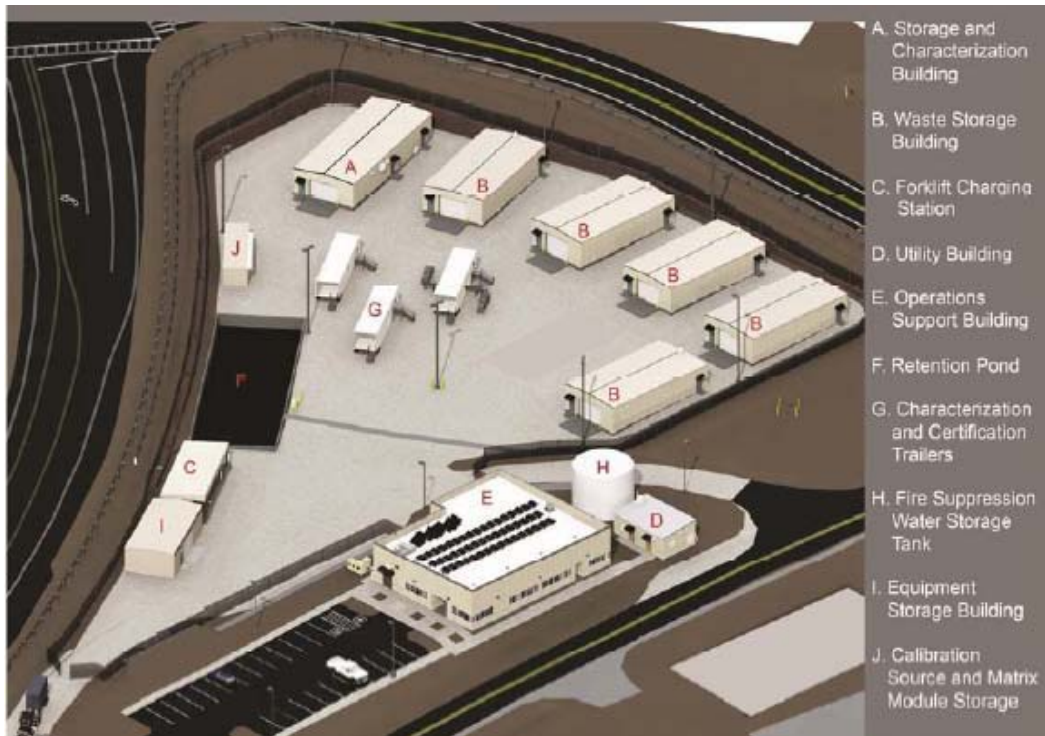
Layout of the Transuranic Waste Facility
