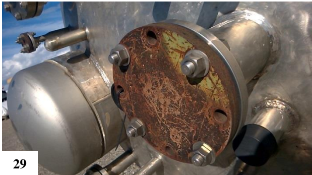
Figures A-26 to A-29. Staff review team photographs illustrating improper segregation of dissimilar metals. Figures A-26 and A-27 show carbon and stainless steel in contact at the Yakima Warehouse. Figure A-28 shows carbon and stainless steel in contact at the High-Level Waste Facility. Figure A-29 shows a carbon steel flange cover on a stainless steel vessel at the WTP construction site
