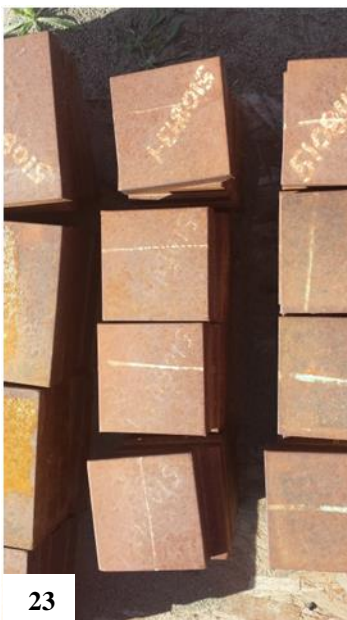
Figures A-23 to A-25. Staff review team photographs illustrating illegible physical markings of SSCs at the MHF Laydown Yard.
