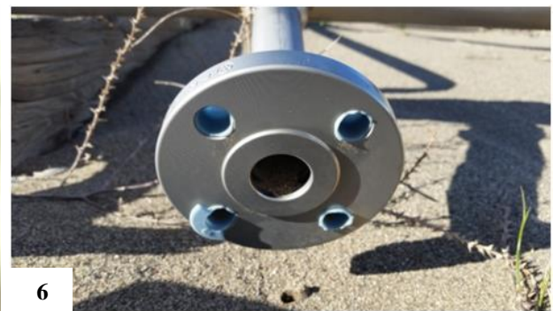
Figures A-1 to A-6. Staff review team photographs illustrating deficient storage conditions at the Material Handling Facility (MHF) Laydown Yard. Figure A-1 shows pipes buried in the sand. Figures A-2, A-4, and A-6 show missing pipe caps on pipe modules and a layer of sand built up inside. Figure A-3 shows excessive vegetation surrounding pipe modules. Figure A-5 appears to show part of an insect nest inside a structure, system, or component (SSC).
