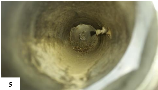
Figures A-1 to A-6. Staff review team photographs illustrating deficient storage conditions at the Material Handling Facility (MHF) Laydown Yard. Figure A-1 shows pipes buried in the sand. Figures A-2, A-4, and A-6 show missing pipe caps on pipe modules and a layer of sand built up inside. Figure A-3 shows excessive vegetation surrounding pipe modules. Figure A-5 appears to show part of an insect nest inside a structure, system, or component (SSC).
