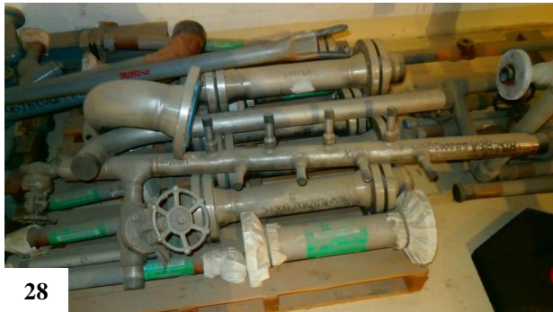
Figures A-26 to A-29. Staff review team photographs illustrating improper segregation of dissimilar metals. Figures A-26 and A-27 show carbon and stainless steel in contact at the Yakima Warehouse. Figure A-28 shows carbon and stainless steel in contact at the High-Level Waste Facility. Figure A-29 shows a carbon steel flange cover on a stainless steel vessel at the WTP construction site
