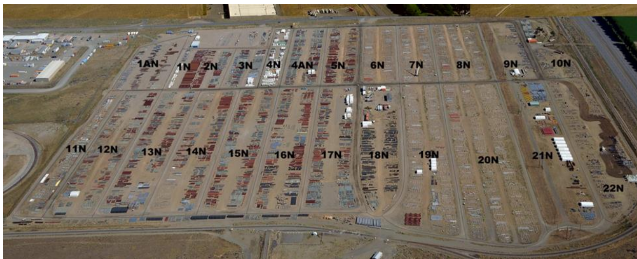
Figure 1. An aerial photograph of the 130 acre MHF Laydown Yard located in Richland, Washington. The MHF Laydown Yard includes 10 miles of roadway, 24 storage rows (labeled in the photograph), 106,154 items, and 15,077 tons of structural steel. Approximately 47 and 50 percent of these SSCs are for the Pretreatment and High-Level Waste Facilities, respectively.
