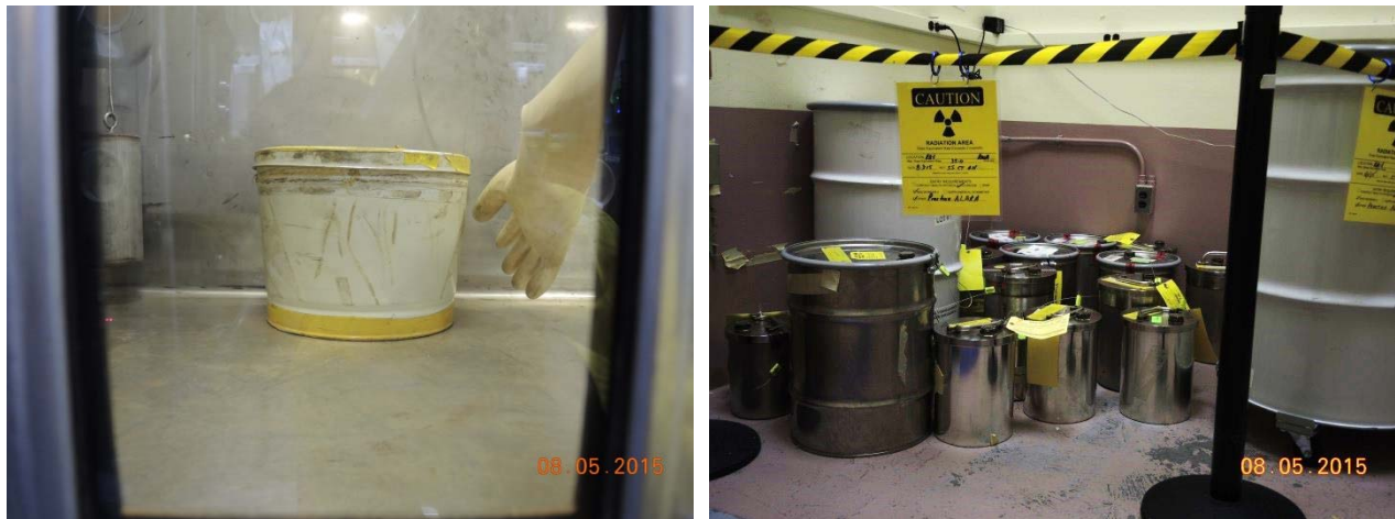
Figure 4: Common MAR storage locations on the first floor of PF-4: a glovebox location holding a legacy “popcorn tin” containing plutonium (left) and one example of a floor storage location (right).
