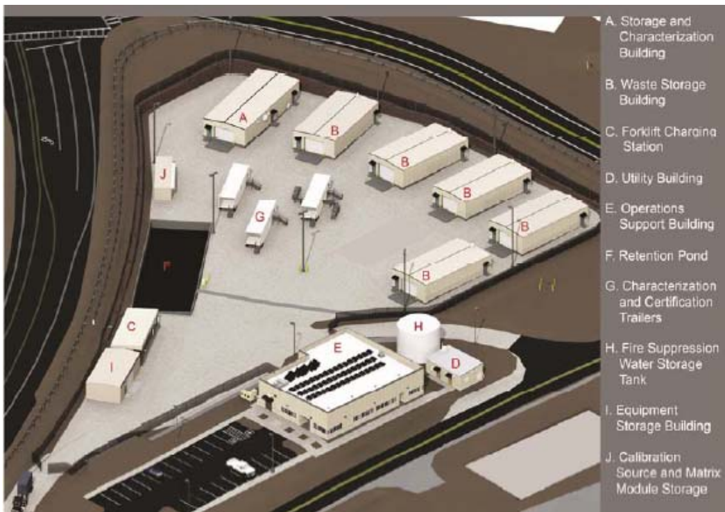
Layout of the Transuranic Waste Facility
