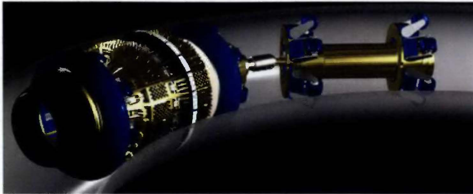
Figure 13: Magnetic Flux Leakage Device in Pipe Bend
