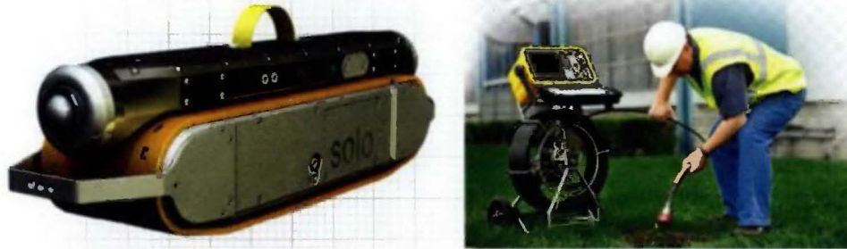
Figure 6: Typical Visual Inspection (ROV - Left, Borescope - Right)
