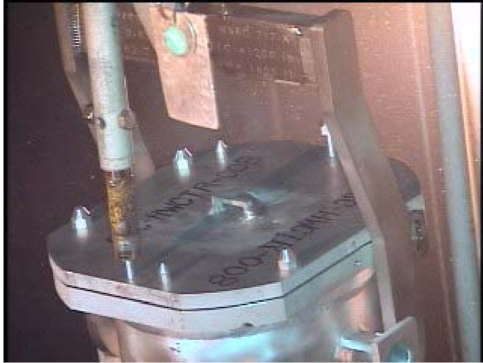
Figure 6. Installing the lid on an L oversized can.
