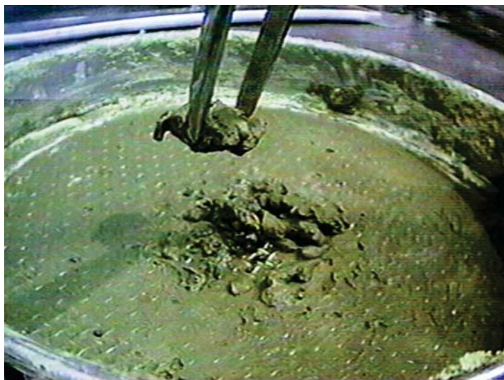
Figure 4-4. Portion of Tank AN-102 Grab Sample Retained on a 2.38 mm Sieve
