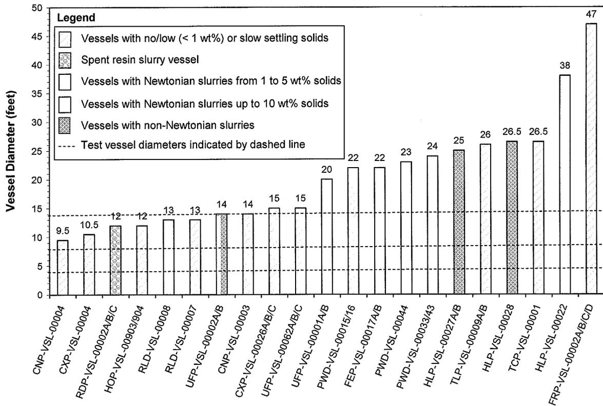
The 14-foot test vessel allows full-scale tests of the UFP-VSL-00002A/B and RLD-VSL-00008 vessels.
