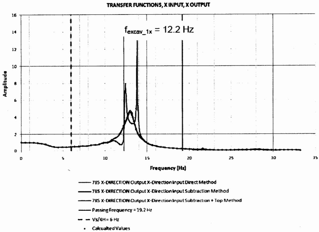
**Figure 41.** Model 3 Transfer Function for 13 Hz Mass, X-Direction
