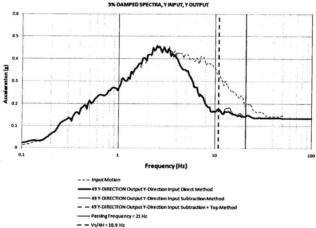
**Figure 25.** Response Spectra for Uniform Soil Case, Coarse Mesh, Y-Direction
