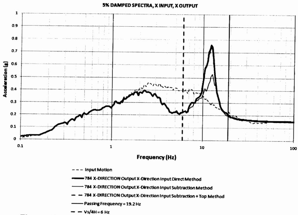
**Figure 40. Model 3 Response Spectra for 12 Hz Mass, X-Direction**
