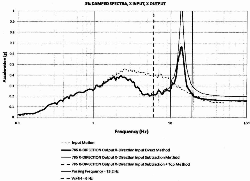
**Figure 44. Model 3 Response Spectra for 14 Hz Mass, X-Direction**
