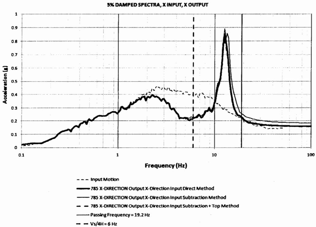
**Figure 42.** Model 3 Response Spectra for 13 Hz Mass, X-Direction
