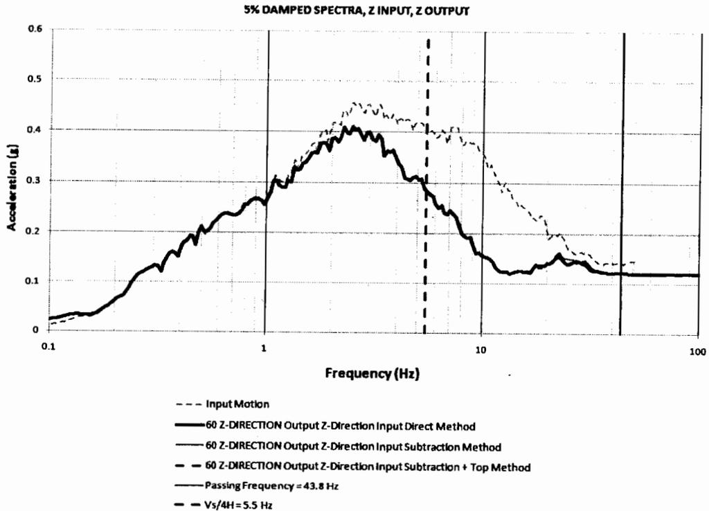
**Figure 11.** Response spectra for Uniform Soil Case, Cube Model, Z-Direction
