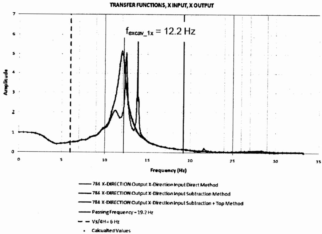
**Figure 39. Model 3 Transfer Function 12 Hz Mass, X-Direction**
