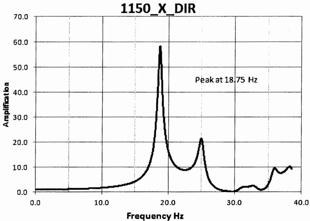
**Figure 15.** First frequency of the constrained box (soil properties for HOUSE model in rigid soil) are about 18.75 Hz for the SASSI transfer function and 18.8 Hz for the GT STRUDL analysis, both with 1350 fps soil
