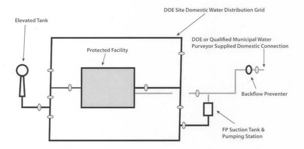
This arrangement could be utilized for SS applications, if conditions specified in A.3.2 and A.3.3. of this standard are met. If the supplied system (e.g., wet pipe sprinkler) needs to operate in a seismic event (e.g., to mitigate a seismically induced fire), the supply system shall be qualified to the same level as the supplied system.
