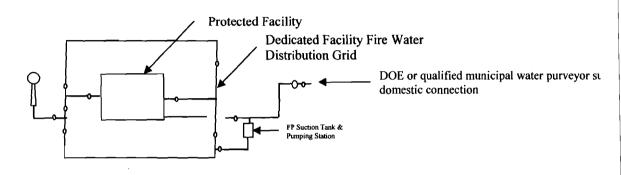
This arrangement could be utilized for safety significant applications if conditions specified in Section 5.3 of this guide are met. If the supplied system (e.g., wet pipe sprinkler) needs to operate in a seismic event (e.g., to mitigate a seismically induced fire), then the supply system must be qualified to the same level as the supplied system.
