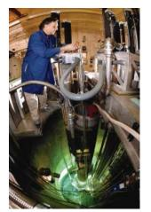
Reactor Operator Checks **Equipment on the Annular** Core Research Reactor, Which Sits at the Bottom of a 30-Foot-Deep Open
