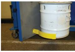
Army/Navy Can Being Inserted Into High **Explosive Transportation Cart**
