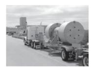
An important WIPP milestone was realized with the delivery of the first Nuclear Regulatory Commission certified RH-72B cask to the site. The cask will be used to transport remote-handled TRU waste to the WIPP for permanent disposal.
