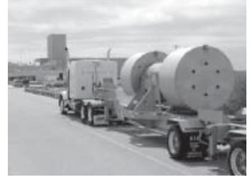
*An important WIPP milestone was realized with the delivery of the first Nuclear Regulatory Commission certified RH-72B cask to the site. The cask will be used to transport remote-handled TRU waste to the WIPP for permanent disposal.*
