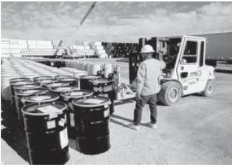
*Drums Containing Low-Level Waste are Unloaded and Staged Prior to Disposal in Pit 8 at the Area 5 Radioactive Waste Management Site Located on NTS.*
