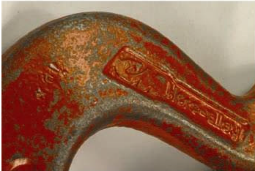
Represented as being new in condition shown Appearance very worn. Is correct manufacturer markings for orange hook.
