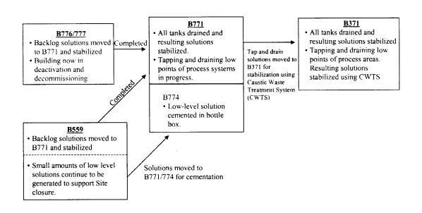
Figure 5.2.3-1: Plutonium Solution Stabilization Process Flow Diagram
