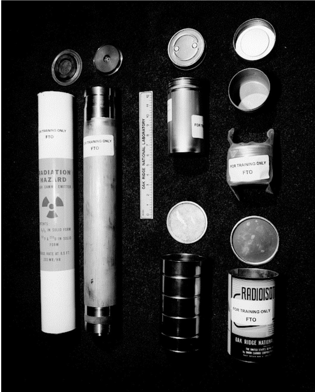
Figure 1. Typical U-233 Storage Containers used in ORNL Building 3019. 3
